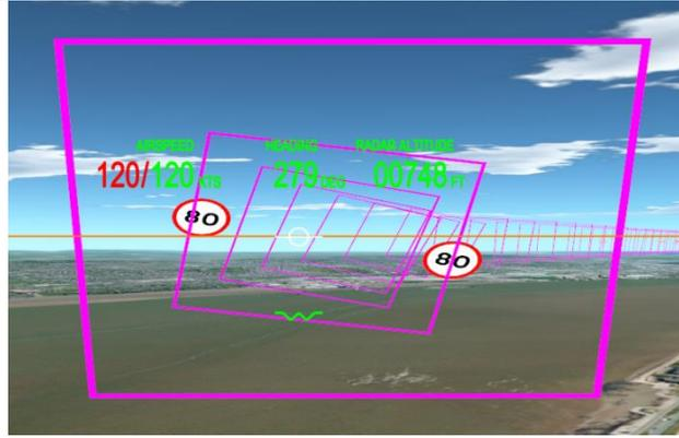
**Figure 6: Highway-n-the-Sky used for PAV Navigation**
