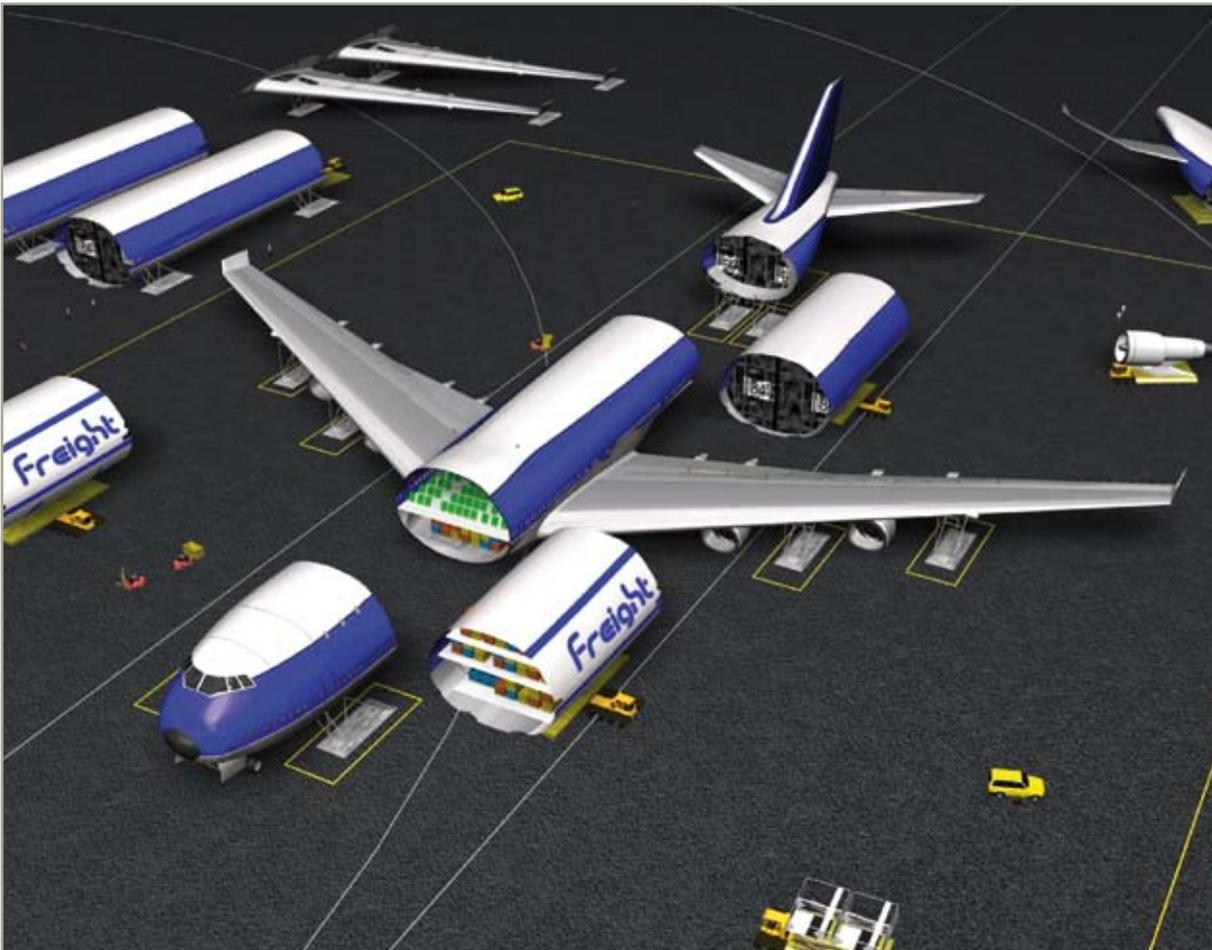
little effect on the aircraft flight characteristics. More fundamental changes to the aircraft have been envisaged. These include pods that may be attached to provide different uses for the aircraft, power-plant change routines, individual passenger enclosures or personal seat units, and wing sets for different duties.
