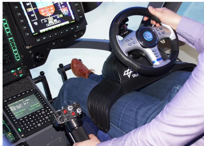
A car-like steering concept in the Flying Helicopter Simulator (Images: DLR)
