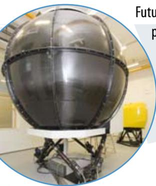
*The HELIFLIGHT-R simulator is used for model validations.*
